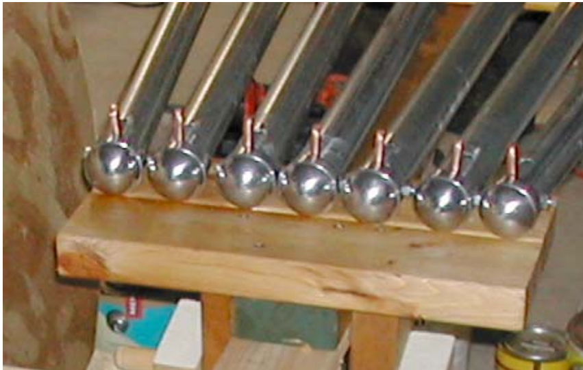
During construction – the barrel caps and drop pins in place.
