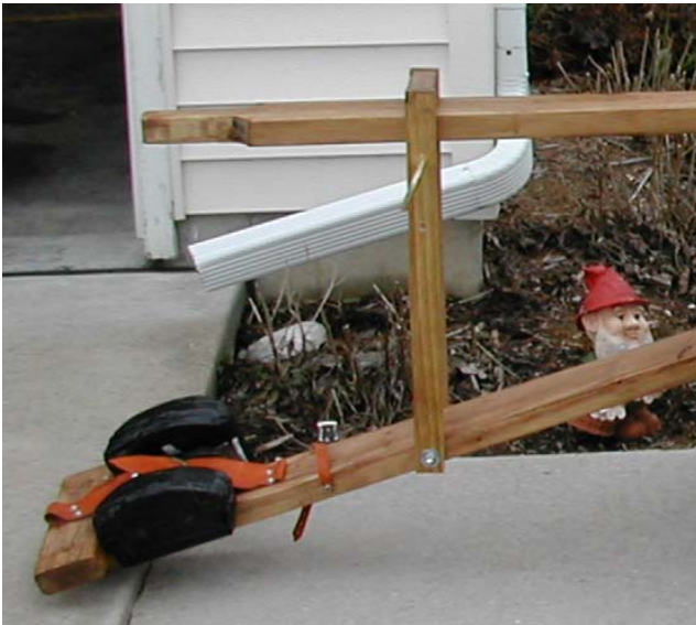
The counterweight strapped on and the elevation set for almost true level ( while the garden gnome looks on... ).
